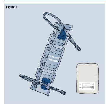
A PFEIFER-VS<sup>®</sup> system, when using VS<sup>®</sup> Slim Boxes, always consists of at least two pairs of boxes opposite each other and a suitable joint filling material. As suitable material, grout or plastic mortar is available to the user. The system is suitable for connecting precast reinforced concrete walls of concrete quality C30/37 and higher.
