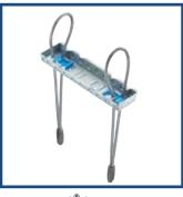
The PFEIFER-VS<sup>®</sup> Slim Boxes Easyfill are used to connect wall-type precast concrete elements. They are able to transmit forces to the connecting joints in all directions and consist of a stable steel plate box suitable for construction, in which the fold-out, flexible wire rope loops are found. Wall joints can be produced inexpensively, easily and safely.
