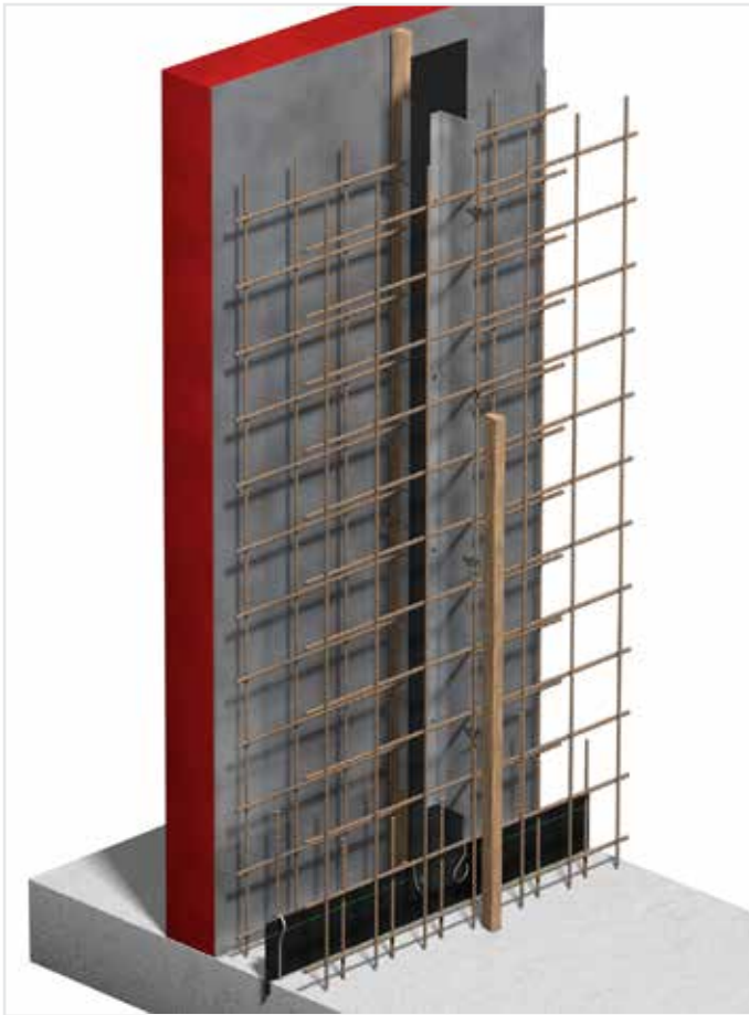
OBS crack control element
