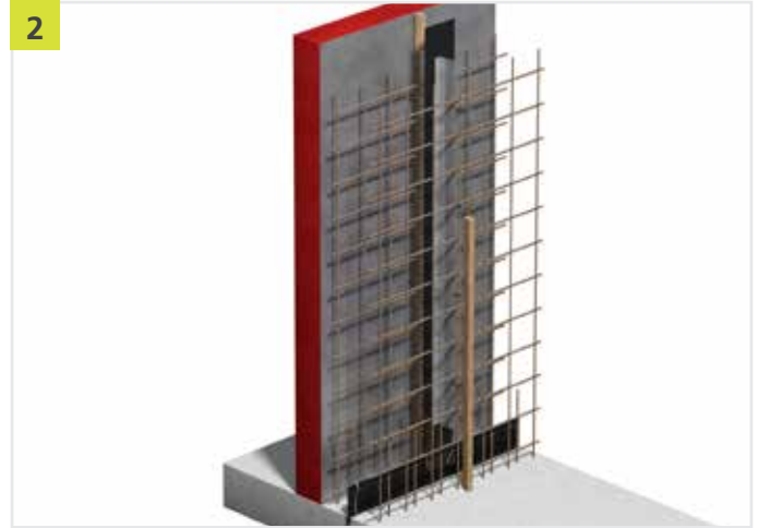
Install a suitable shuttering of size c_{nom} into the formwork at the exact point where the predetermined crack ought to form (level of the assembly sheet steel).
