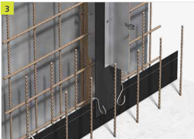
Install the OBS element in the wall formwork between the outer and inner reinforcement layers. Tie wire is used to attach it. Thread the wire through the holes provided in the assembly sheets and fix tie to the reinforcement. The position of the OBS element must be fixed so that the assembly sheet steel is immovable at the level of the planned pre-break point; this means that the sealing plane will be exactly parallel with the surface of the formwork on the axis of the floor/wall joint seal.
