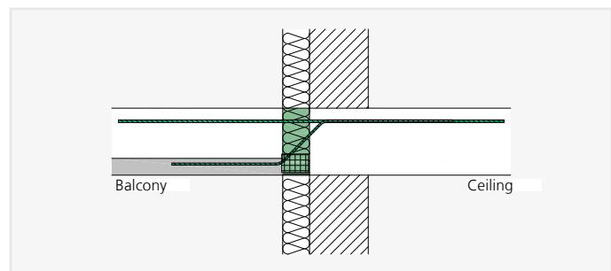
ISOPRO® A-IP two-part – Installation cross-section thermal insulation composite system
