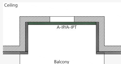
ISOPRO® A-IP/A-IPT – Cantilevered balconies in façade recesses
