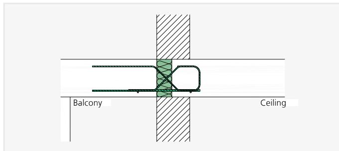
ISOPRO® A-IPTQQ – Installation cross-section of single-leaf masonry – shear rod on the ceiling, looped
