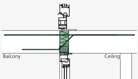
ISOPRO® A-IP – Installation cross-section for glass façades
