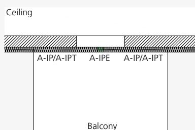
ISOPRO® A-IPE – Cantilevered balcony with lifting moments
