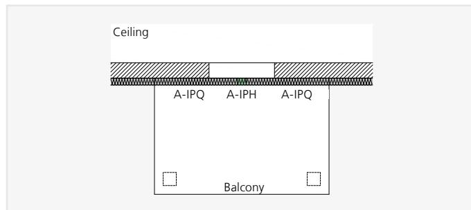
ISOPRO® A-IPH – Balcony on hinged supports with A-IPH structural units
