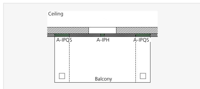
ISOPRO® A-IPQS – Supported balcony with beams and support at specific points with ISOPRO® A-IPQS units
