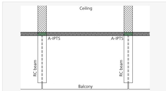
ISOPRO® A-IPTS – Balcony structure with prefabricated slabs joined by a non-static connection, and load-carrying joists
