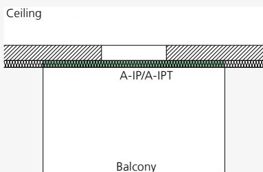
ISOPRO® A-IP/A-IPT – Cantilevered balconies
