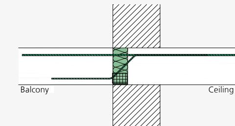
ISOPRO® IP – Installation cross-section for single-leaf masonry
