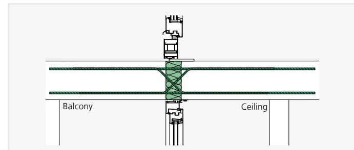
ISOPRO® A-IPTD – Installation cross-section of glass façade
