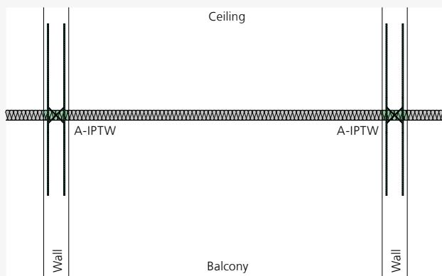
ISOPRO® A-IPTW – Arrangement of units in the floor plan in combination with a balcony slab
