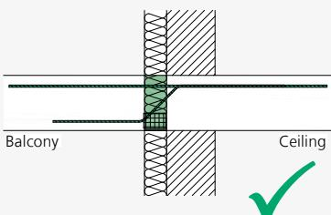
ISOPRO® IP – Correct installation
