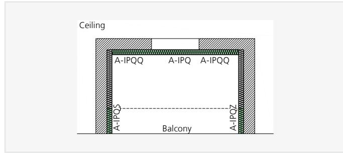
ISOPRO® A-IPQ, A-IPQQ, A-IPQS, A-IPQZ – Loggia balcony with load peaks at specific points and constraint-free support at the front
