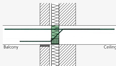
ISOPRO® A-IP – Installation cross-section for double leaf masonry
