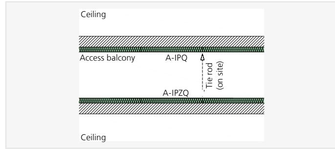
ISOPRO® A-IPQ, A-IPZQ – Access balcony with constraint-free support
