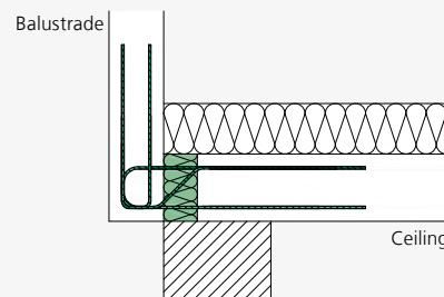
ISOPRO® A-IPTF – Installation cross-section of a balustrade connected to the vertical face with thermally insulating masonry
