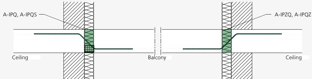
ISOPRO® A-IPQ/A-IPZQ , A-IPQS/A-IPQZ – Installation cross-section with opposite types of same load bearing capacity
