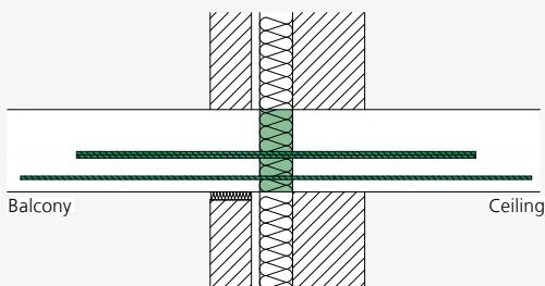
ISOPRO® A-IPE – Installation cross-section of two-leaf masonry
