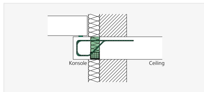
ISOPRO® A-IPO – Corbel as support for a prefabricated component, support with centring bearing
