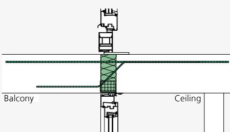
ISOPRO® IP – Installation cross-section for glass façade
