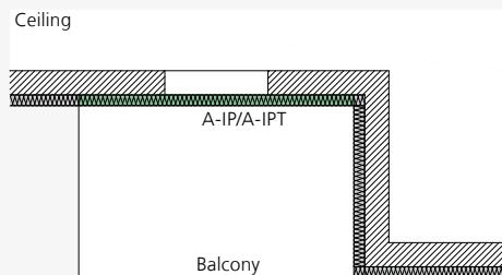
ISOPRO® A-IP/A-IPT – Cantilevered balconies in façade extensions
