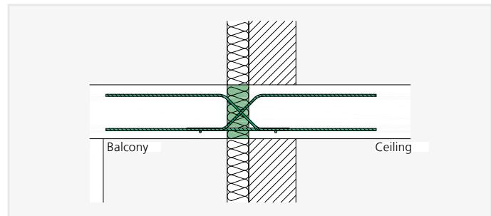
ISOPRO® A-IPTQQ, A-IPTQQS – Installation cross-section of thermal insulation composite system – shear rod on the ceiling, straight
