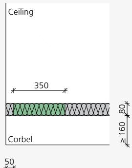
The following distances must be maintained around the edges of ceilings or balustrades and around expansion joints:
