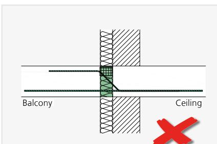
ISOPRO® IP – Incorrect installation, tension rod must be at the top
