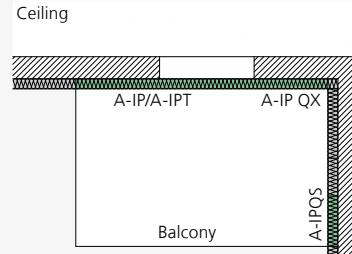
ISOPRO® A-IP/A-IPT in combination with A-IP QX and A-IPQS for internal corner balconies
