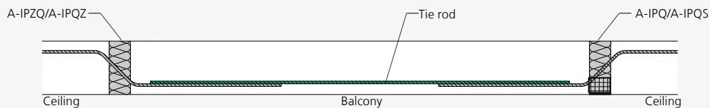
ISOPRO® A-IPZQ/A-IPQ, A-IPQZ/A-IPQS – On-site tie rod in the bottom layer of reinforcement – Shear rod on the ceiling, straight
