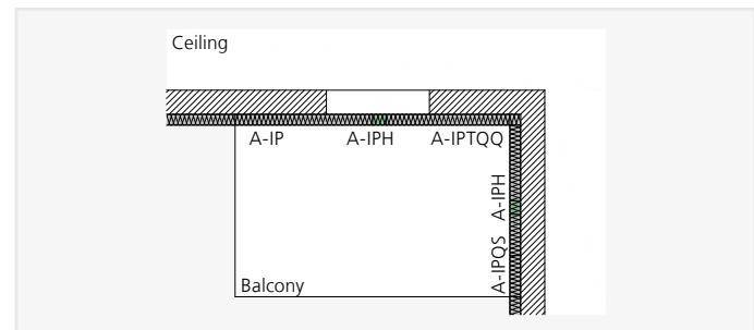
ISOPRO® A-IPH – Supported internal corner balcony with planned horizontal loads
