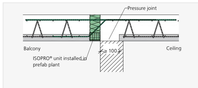
ISOPRO® A-IP – Pressure joint for prefabricated slabs on the ceiling
