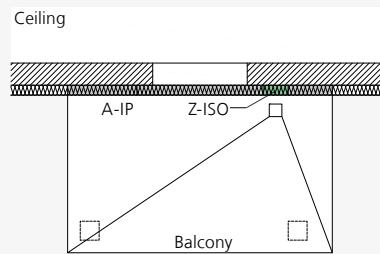
ISOPRO® Z-ISO – Balcony on supports – Z-ISO units in the drainage recess area
