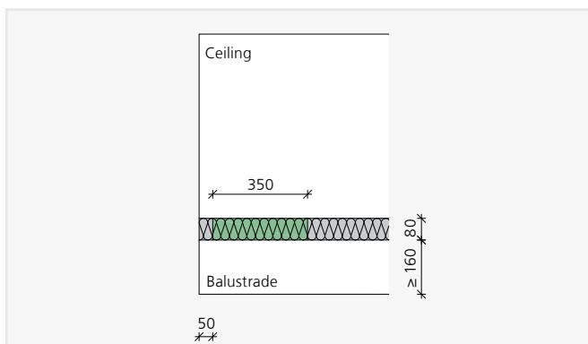
The following distances must be maintained around the edges of ceilings or balustrades and around expansion joints
