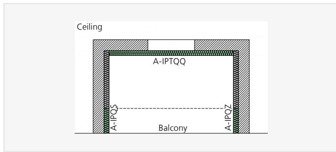
ISOPRO® A-IPTQQ, A-IPQS, A-IPQZ – Loggia balcony with load peaks at specific points at the front and lifting loads in the rear corner area
