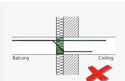
ISOPRO® IP – Incorrect installation, shear rod must be on the bottom side of the balcony
