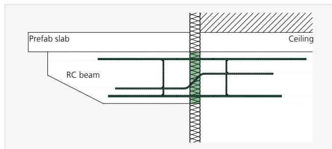
ISOPRO® A-IPTS – Installation cross-section with prefabricated slabs
