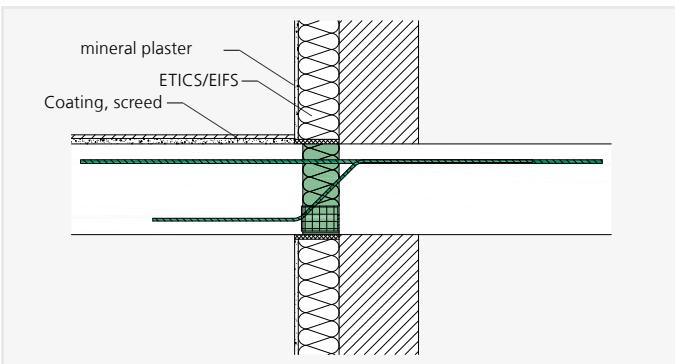
REI120 embedment of ISOPRO® unit im thermal insulation composite system
