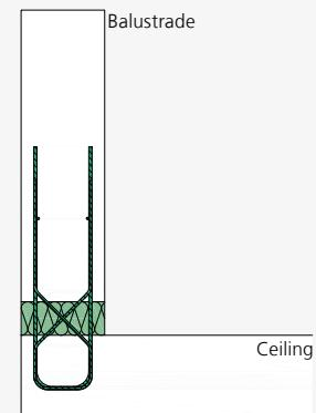
ISOPRO® A-IPTA – Installation cross-section of balustrade connected to the horizontal face
