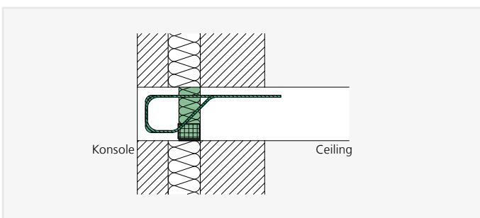
ISOPRO® A-IPO – Corbel with facing masonry
