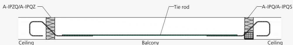
ISOPRO® A-IPZQ/A-IPQ, A-IPQZ/A-IPQS – On-site tie rod in the bottom layer of reinforcement – Shear rod Ø 6 on the ceiling, looped
