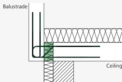
ISOPRO® A-IPTF – Installation cross-section of a balustrade connected to the vertical face with a thermal insulation composite system
