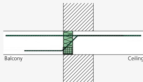
ISOPRO® A-IP – Installation cross-section for single-leaf masonry
