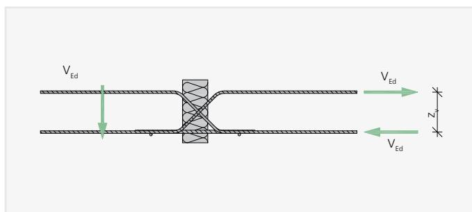
ISOPRO® A-IPTQQ, A-IPTQQS – Units with steel pressure rods
