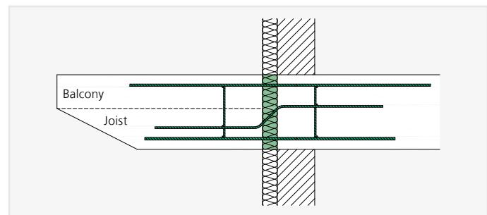
ISOPRO® A-IPTS – Installation cross-section with joists connected to the balcony slab monolithically
