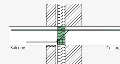
ISOPRO® IP – Installation cross-section for double leaf masonry
