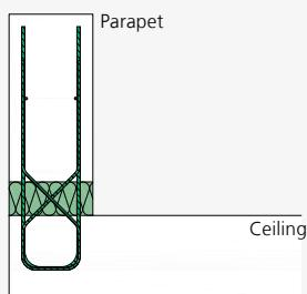
ISOPRO® A-IPTA – Installation cross-section of parapet
