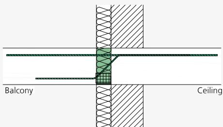
ISOPRO® A-IP – Installation cross-section for external thermal insulation composite system
