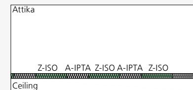
ISOPRO® Z-ISO – Use of parapet units at specific points
