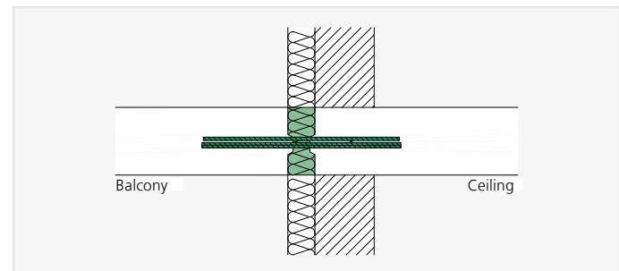
ISOPRO® A-IPH 3 – Installation cross-section of thermal insulation composite system
