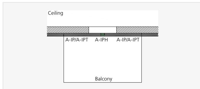
ISOPRO® A-IPH – Cantilevered balcony with planned horizontal loads
