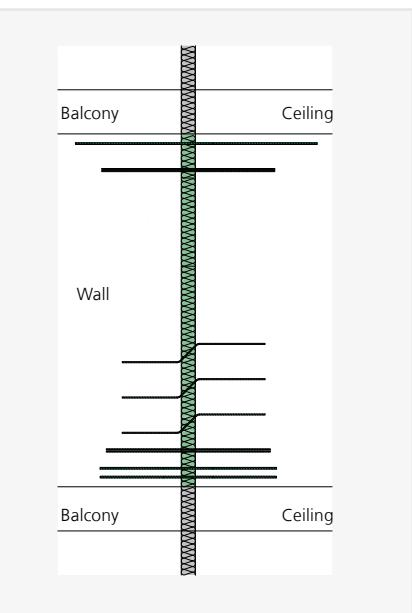
ISOPRO® A-IPTW – Installation cross-section with wall slab connected to the balcony slab monolithically
