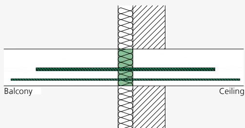
ISOPRO® A-IPE – Installation cross-section of thermal insulation composite system
