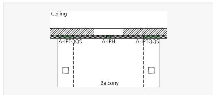
ISOPRO® A-IPTQQS – Supported balcony with joists and support at specific points with ISOPRO® A-IPTQQS units
