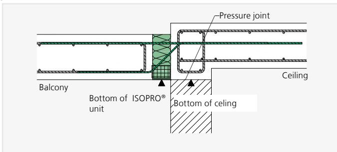
ISOPRO® A-IP – Pressure joint for in-situ concrete construction and vertically offset slabs
