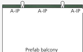
ISOPRO® Z-ISO – Balcony as prefabricated component with transport anchor – the Z-ISO units are added on site
