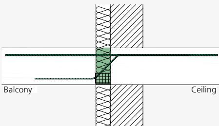
ISOPRO® IP – Installation cross-section for external thermal insulation composite system
