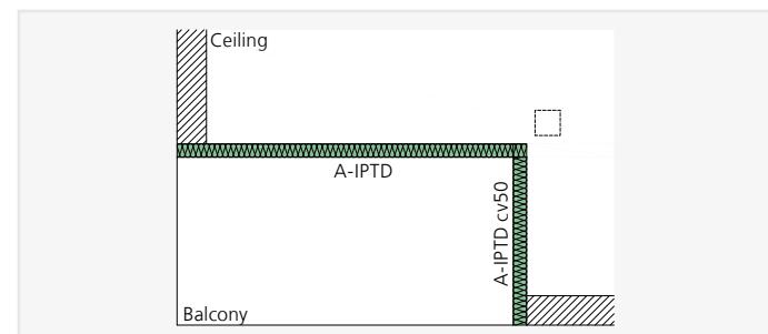
ISOPRO® A-IPTD – Internal corner balcony with large dimensions and loads
