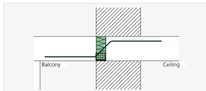
ISOPRO® A-IPQ, A-IPQS – Installation cross-section of single-leaf masonry
