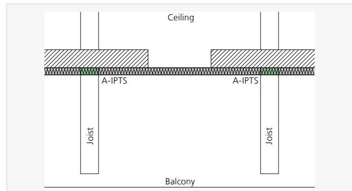
ISOPRO® A-IPTS – Balcony structure with joists connected to the balcony slab monolithically
