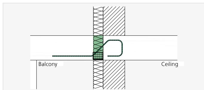
ISOPRO® A-IPQ, A-IPQS – Installation cross-section of thermal insulation composite system
