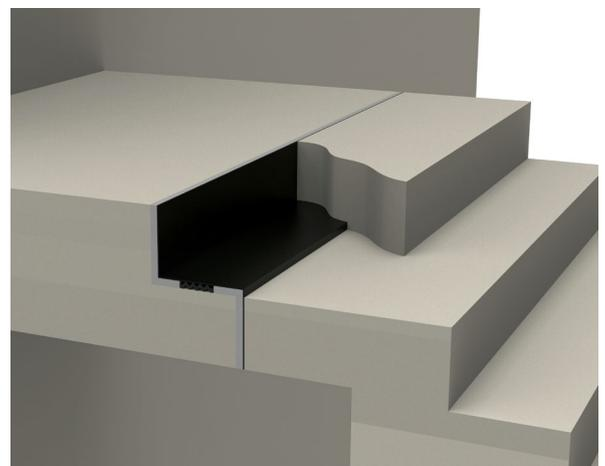
In the case of cast-in-place concrete, the bearing should be installed, so that the cover faces upwards.
